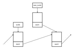
After the line no. 4 of the add\_in\_middle\_or\_at\_back() function is performed
