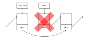
After performing the 6th line of the delete\_middle\_or\_last\_node() function
