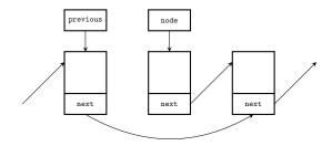
After performing the 5th line of the delete\_middle\_or\_last\_node() function
