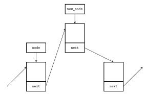
After the line no. 5 of the add\_in\_middle\_or\_at\_back() function is performed
