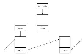
Before the line no. 4 of the add\_in\_middle\_or\_at\_back() function is performed
