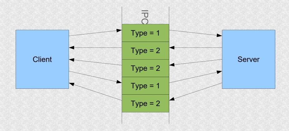
By using message types, two-way communication for the server and multiple clients can be achieved.
